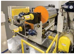
Sheet Take-Off System in retracted open position for access to downstream side of the primary roll stand (PTi Patent No. 7,165,962 B2).
